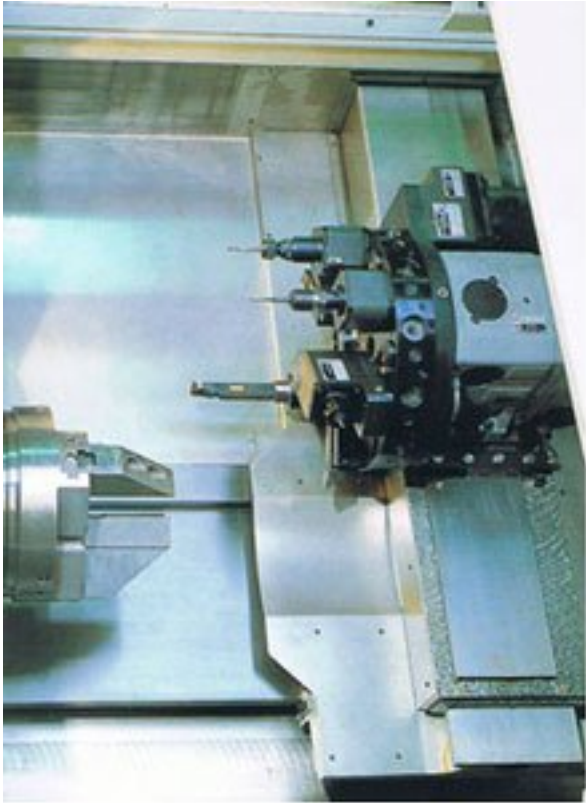
Turret unit with motorized tool-holders
